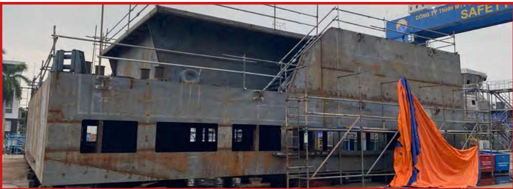
Units 12, 13 and 20 , the aft part of the passenger lounges, have been integrated together and outfitting of this megablock is ongoing, with the installation of pipes, mooring equipment and ventilation ducts. This megablock is on the dockside and will be erected with the rest of the hull once integration of units 4 and 5 is complete.
