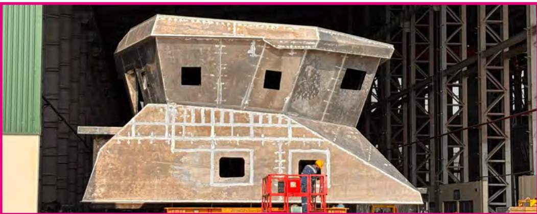
The wheelhouse and upper accommodation aluminium unit ( unit 26 ) is erected with integration to unit 23.1 ongoing. (photo is pre-intergration)
